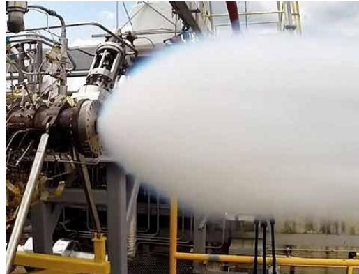
Pintle Injector Cold flow Testing for SpaceX's Raptor engine.
